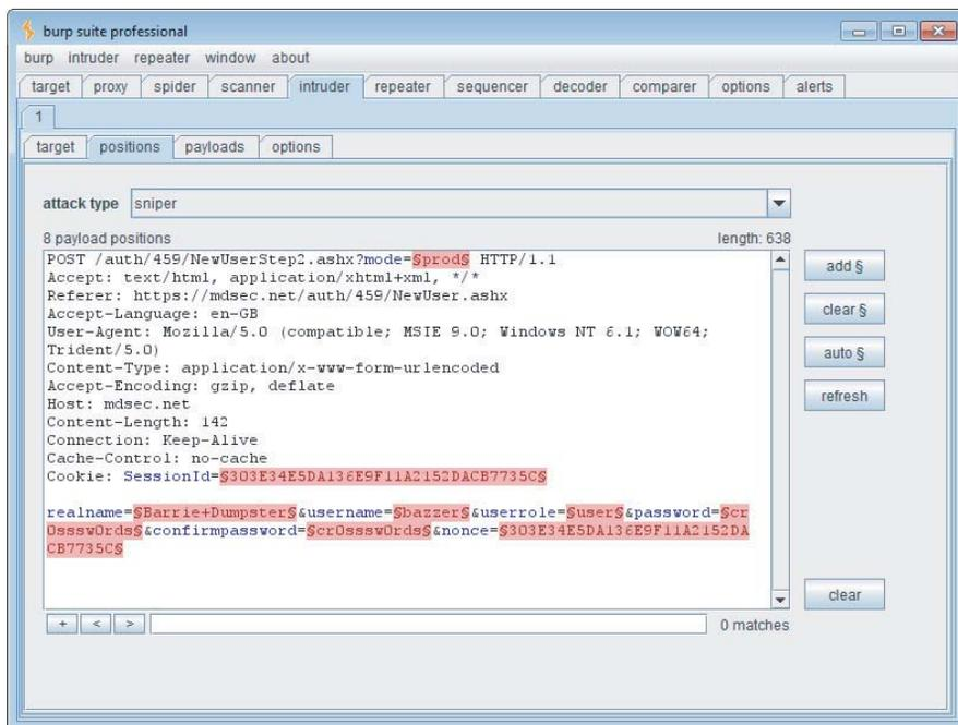
**Figure 14-1:** Positioning payloads
