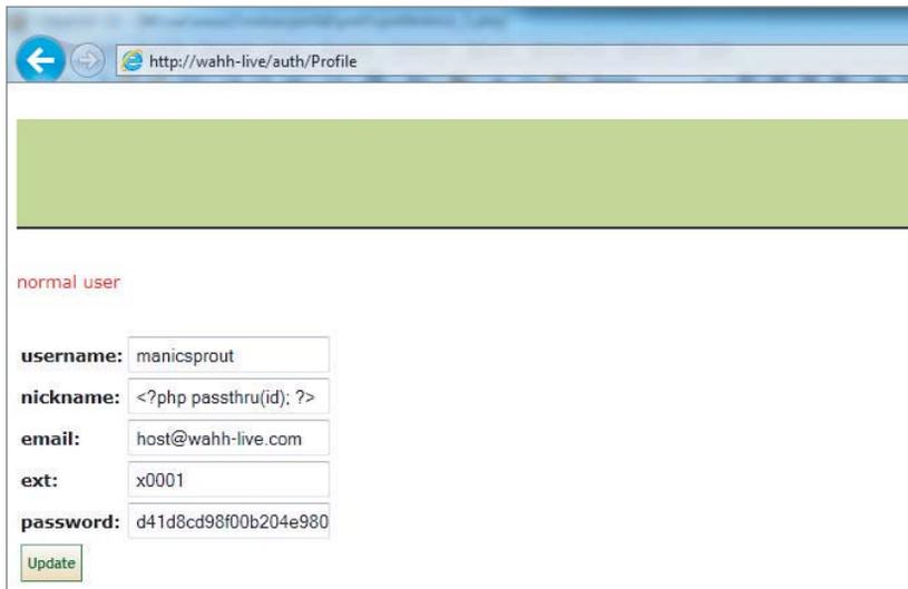
**Figure 17-3:** Configuring a nickname containing server-executable script code
