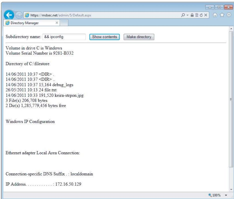
**Figure 10-4:** A successful command injection attack
